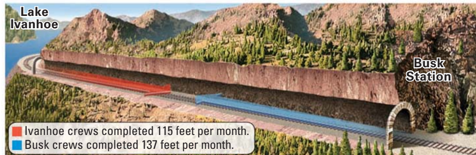
Cutaway of Busk-Ivanhoe Tunnel
